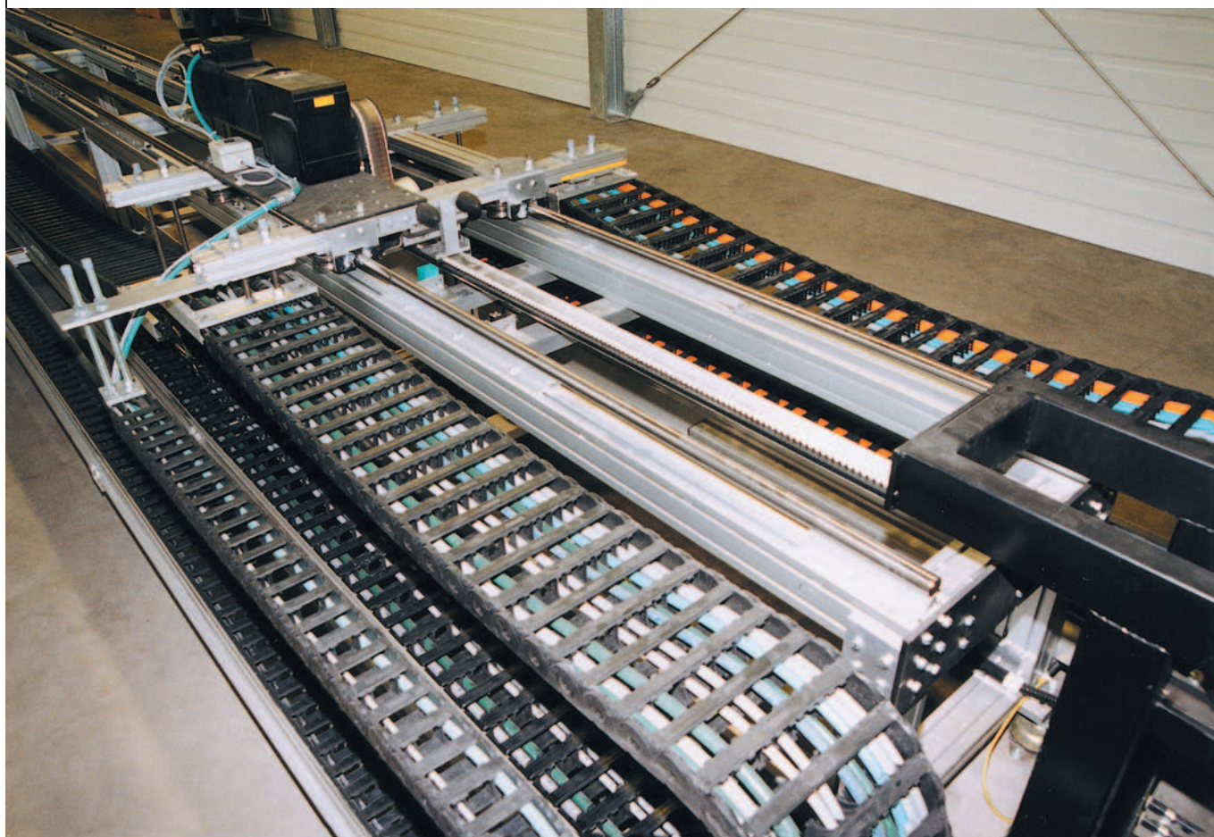
Partial view of drag chain test centre in factory Windsbach
