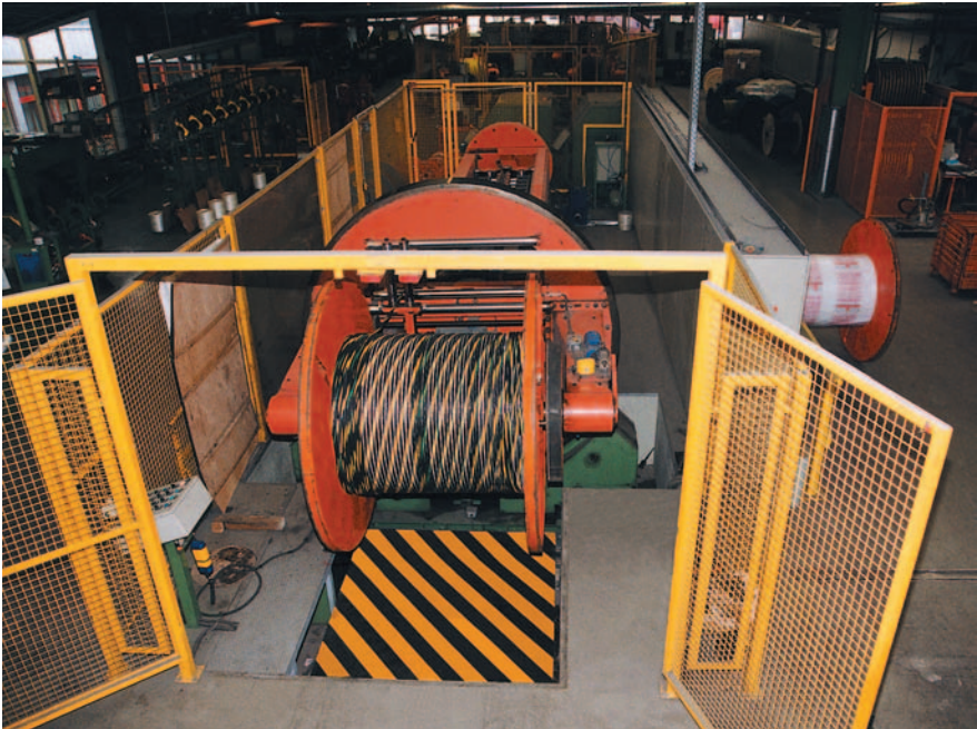
Big stranding machine for cable lay up to 4 x 185 mm² in factory Windsbach. Works photo: HELUKABEL®
